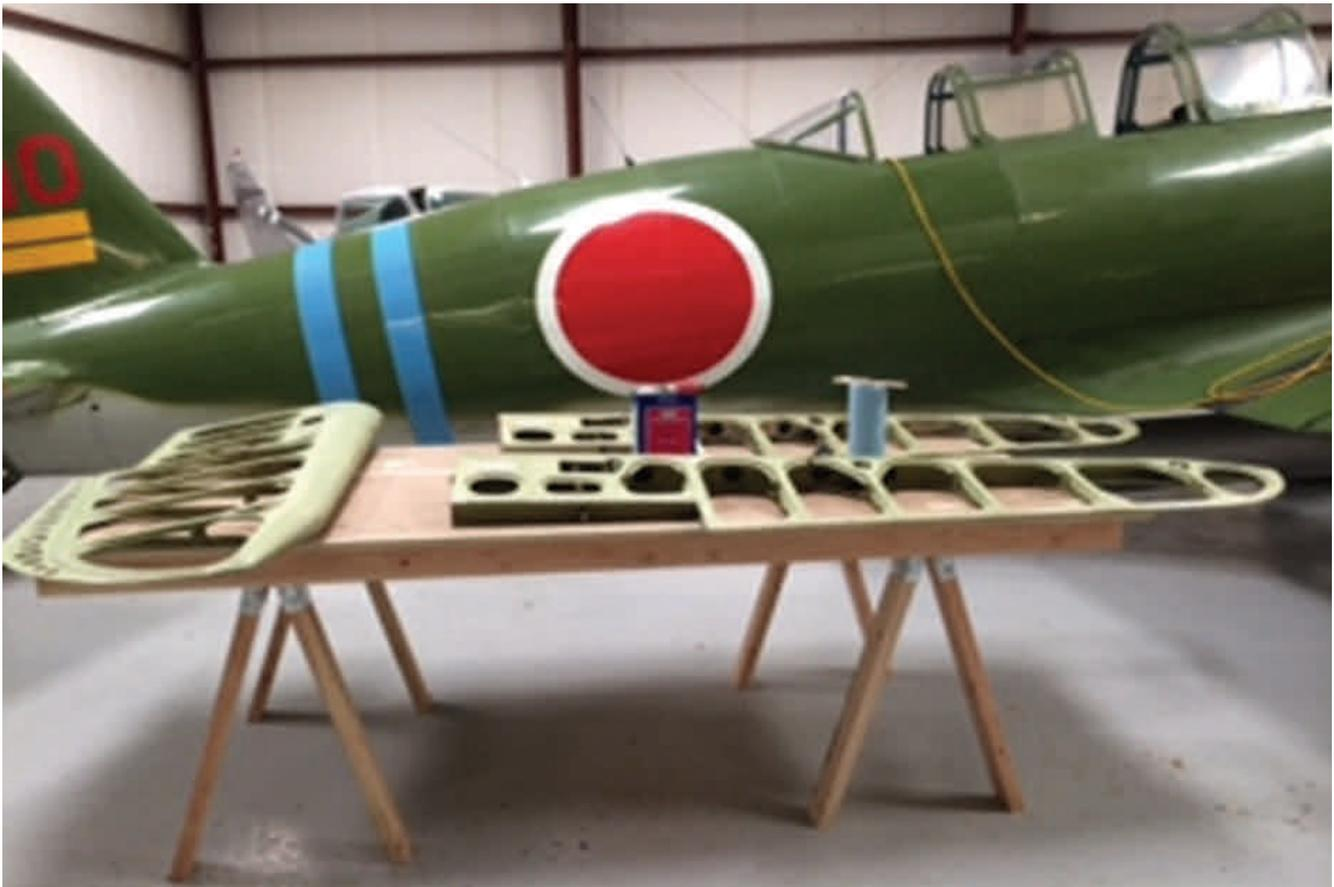
The Kate is presently down for another condition inspection. Generally, we found nothing of concern in the aircraft, but the control surfaces have now been removed, stripped, painted, and are being prepared for recovering.
